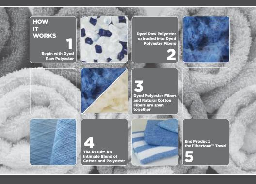
Polyester is solution dyed in its raw state and extruded into fibers. These polyester fibers are then ring spun with cotton fibers to produce an intimate blend. This strategic blend produces a stable and consistent colored yarn. The overall presence of polyester extends the life expectancy of towels with stronger selvages and less linting.
